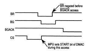
This timing diagram shows that the BR is negated too early and may cause a bus contention between the MPU and DMAC. The problem occurs in the following conditions:
